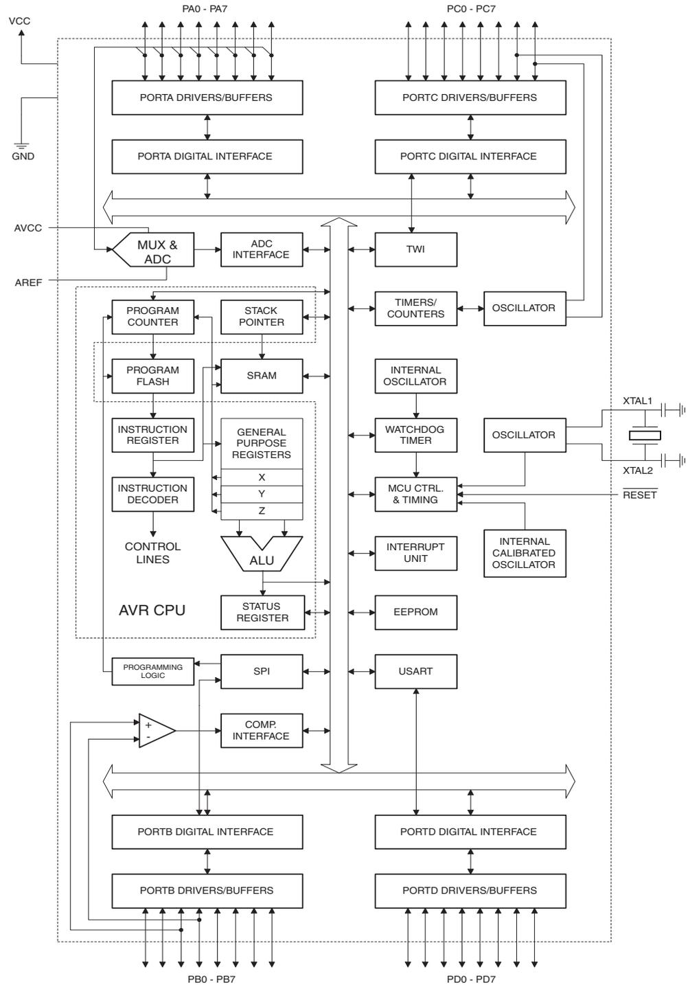
The Atmel® AVR® core combines a rich instruction set with 32 general purpose working registers. All the 32 registers are directly connected to the Arithmetic Logic Unit (ALU), allowing two independent registers to be accessed in one single instruction executed in one clock cycle. The resulting architecture is more code efficient while achieving throughputs up to ten times faster than conventional CISC microcontrollers.
